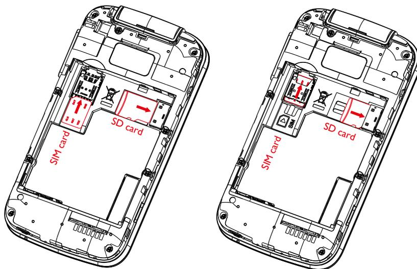
To remove the SIM card or microSD™ card, press down on the small plastic tab (①), then slide out the card (②). Do not use force or use any sharp objects.
