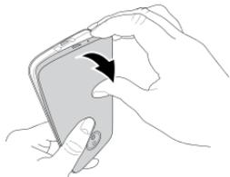
**Caution:** Do not pull the USB port part to remove the back cover.
